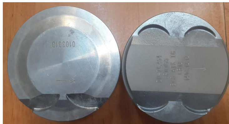
Figure 9 Piston CR 9.5:1 (left) and piston CR 12:1 (right)
