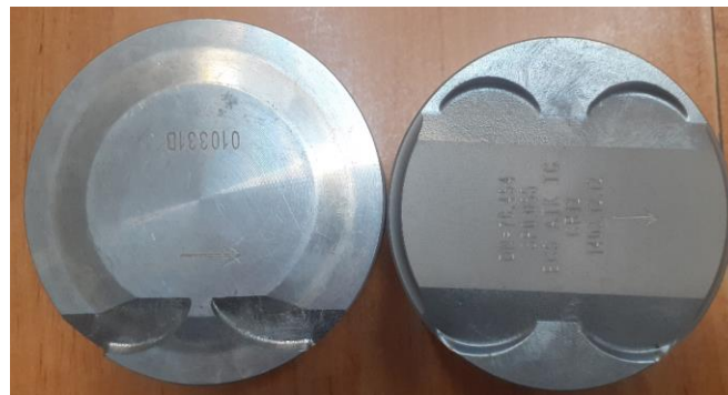
Figure 3 Piston with a compression ratio of 9.5 (left) and a compression ratio of 12 (right)
