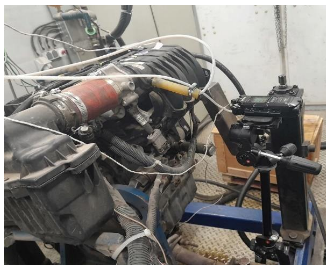
Figure 4 Installing the recorder in front of the intake manifold
