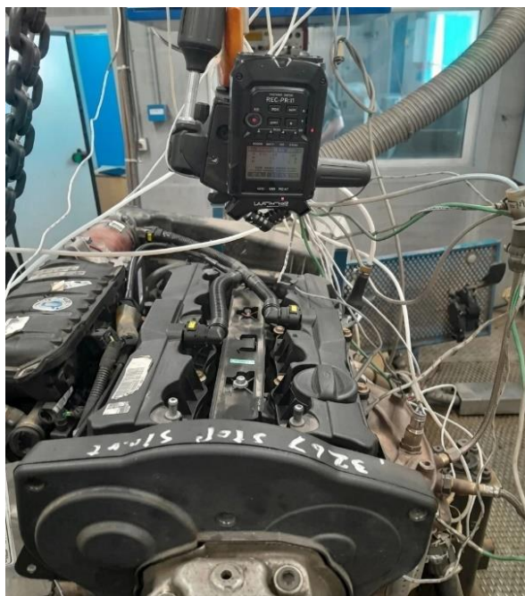
Figure 3 Installing the recorder on top of the engine
