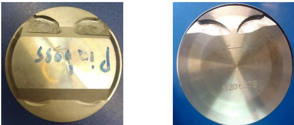
Figure 1 Atkinson Cycle Piston – CR 12.4 (left) - Otto Cycle Piston – CR 10.7 (Right)
