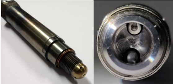
Figure 1: HSASI ignition element (left side) and insight into the pre-chamber with spark plug and glow plug (right side)
