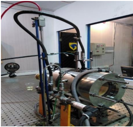
Figure 2: Constant volume test chamber and apparatus set-up
