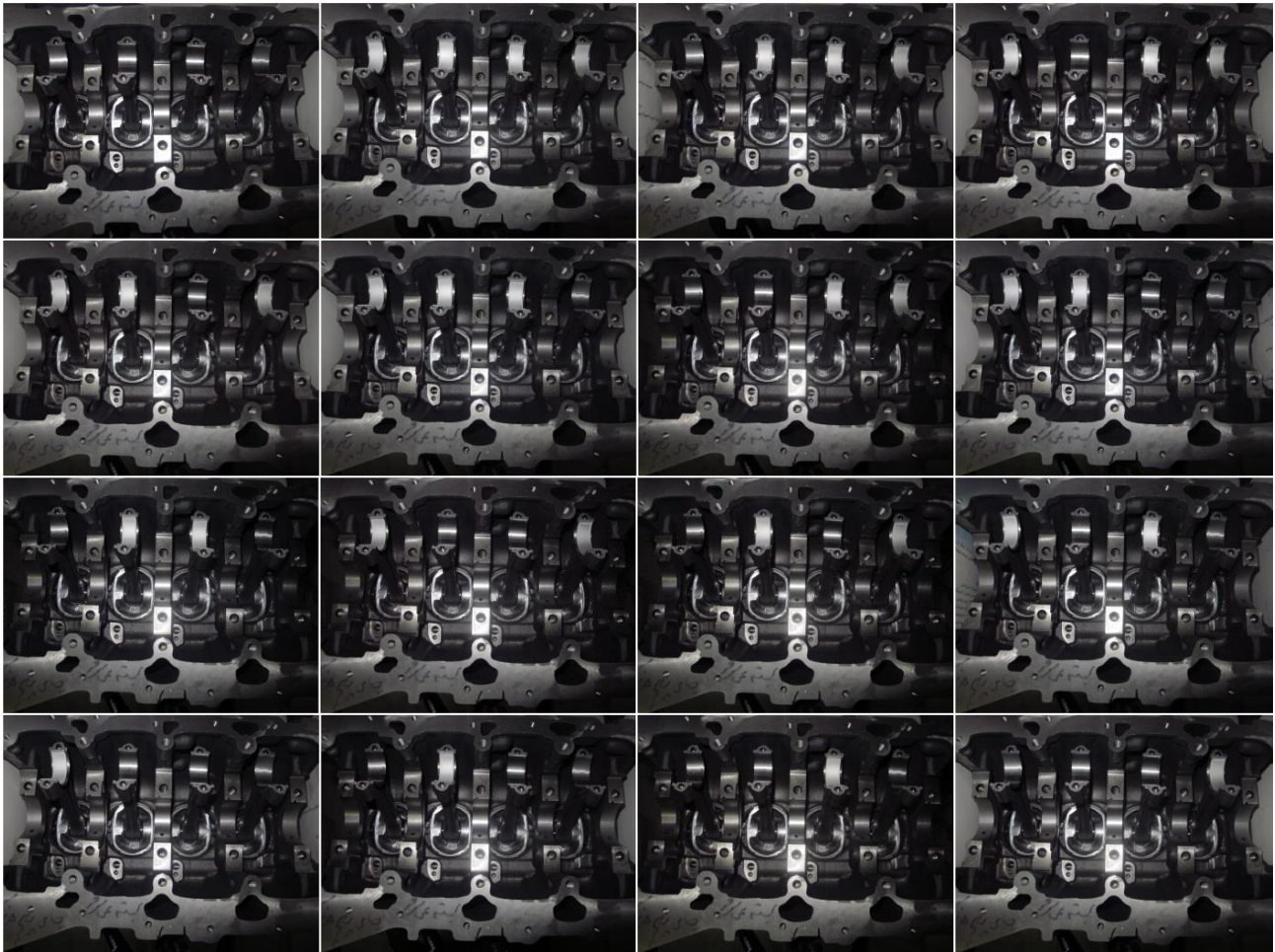
Figure 3: 16 different cases of conrod bearing installation captured by camera
