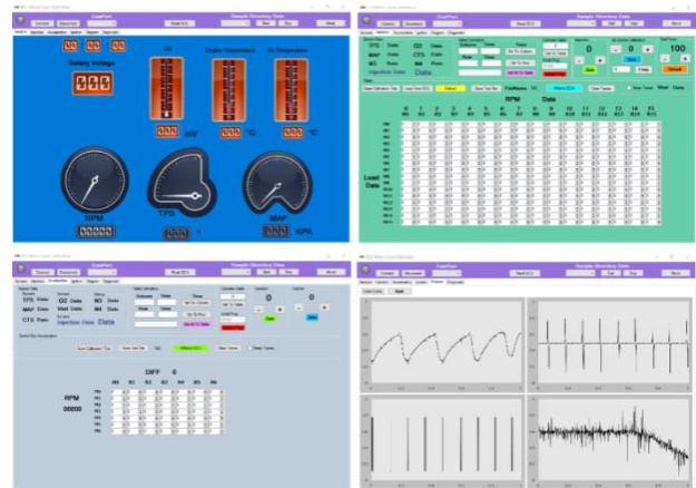
Figure 13: Communicating software with the engine management unit
