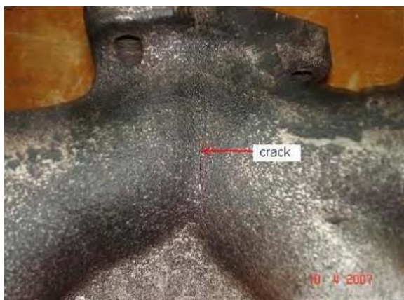
Figure 9: The cracked exhaust manifold [25]
