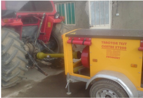
Figure 2: Tractor and Dynamometer setup
