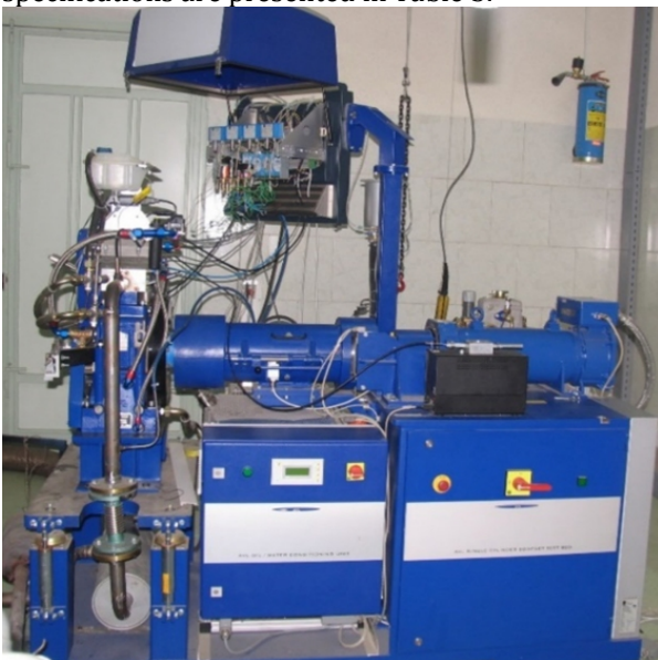
Figure 11: Single cylinder research engine compact test bed of university of Tehran, reference [27]
