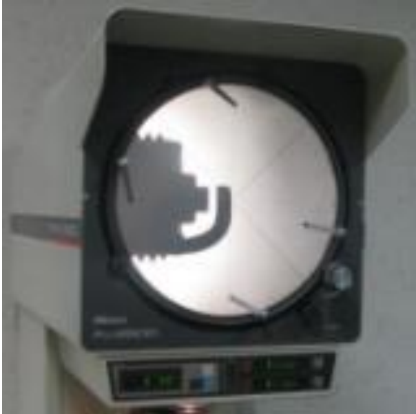
Figure 3: The profile projection of the spark plug electrode
