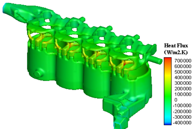
Fig 14. Heat flux distribution on cylinder block coolant jacket
